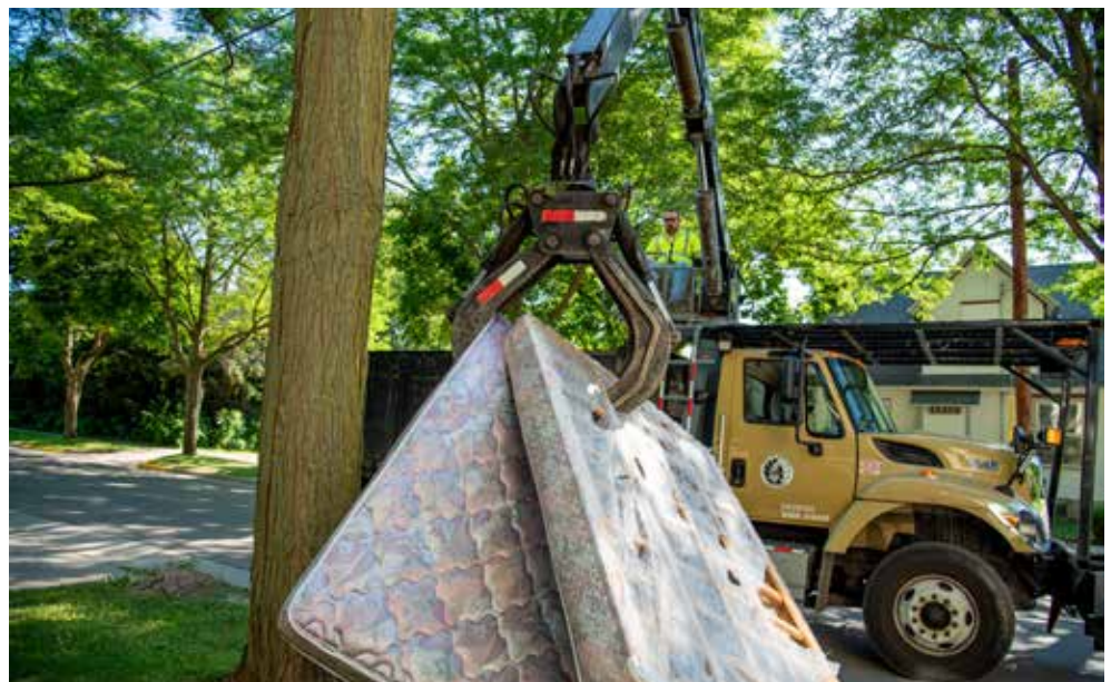
Collecting a mattress & box spring with a truck-mounted crane.
